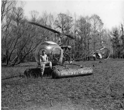
initially supplied a Bell 47B — registration NC21H — with four-wheeled landing gear. (The gear was later changed to floats for landing in the marshes.)
