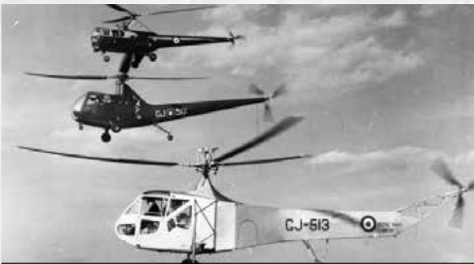
Three British Sikorsky helicopters from the Airborne Forces Experimental Establishment at RAF Beaulieu in Hampshire. Phil Fillingham flew in all three Sikorsky types. From top: Sikorsky S-51; R-4; R-6. Phil Fillingham Collection Photo
