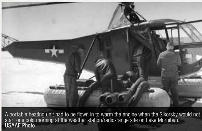
A portable heating unit had to be flown in to warm the engine when the Sikorsky would not start one cold morning at the weather station/radio-range site on Lake Morhiban. USAAF Photo
