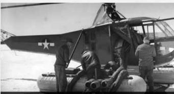
A portable heating unit had to be flown in to warm the engine when the Sikorsky would not start one cold morning at the weather station/radio-range site on Lake Morhiban. USAAF Photo
